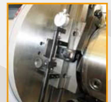
Stroke comparator reduces journal set-up time
