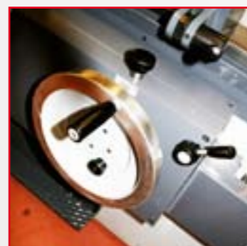
GRINDING WHEEL CONTROL Push button for fine feed Zero stop for fine feed Scale ring for fine feed Locking handle for scale ring Handwheel for grinding wheel fine feed
