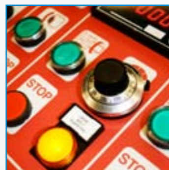
CONTROL PANEL Infinitely adjustable workpiece speeds extend grinding wheel life
