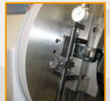
Stroke comparator reduces journal set-up time
