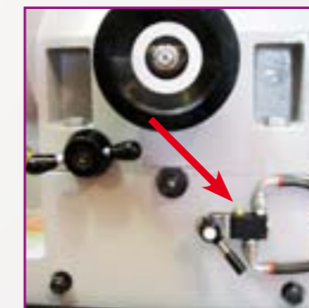
Air cushion system for head displacement
