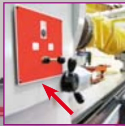
Air cushion system for head displacement
