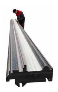
**COMPOSITAL®** a new solution composed by resine-granite mixture filled on welded-steel casing that permits to:
