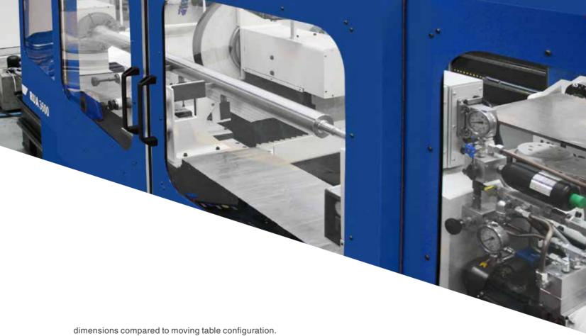
dimensions compared to moving table configuration. Base is in composite material specifically designed to obtain the best result between structural deformations and vibration dumping.
