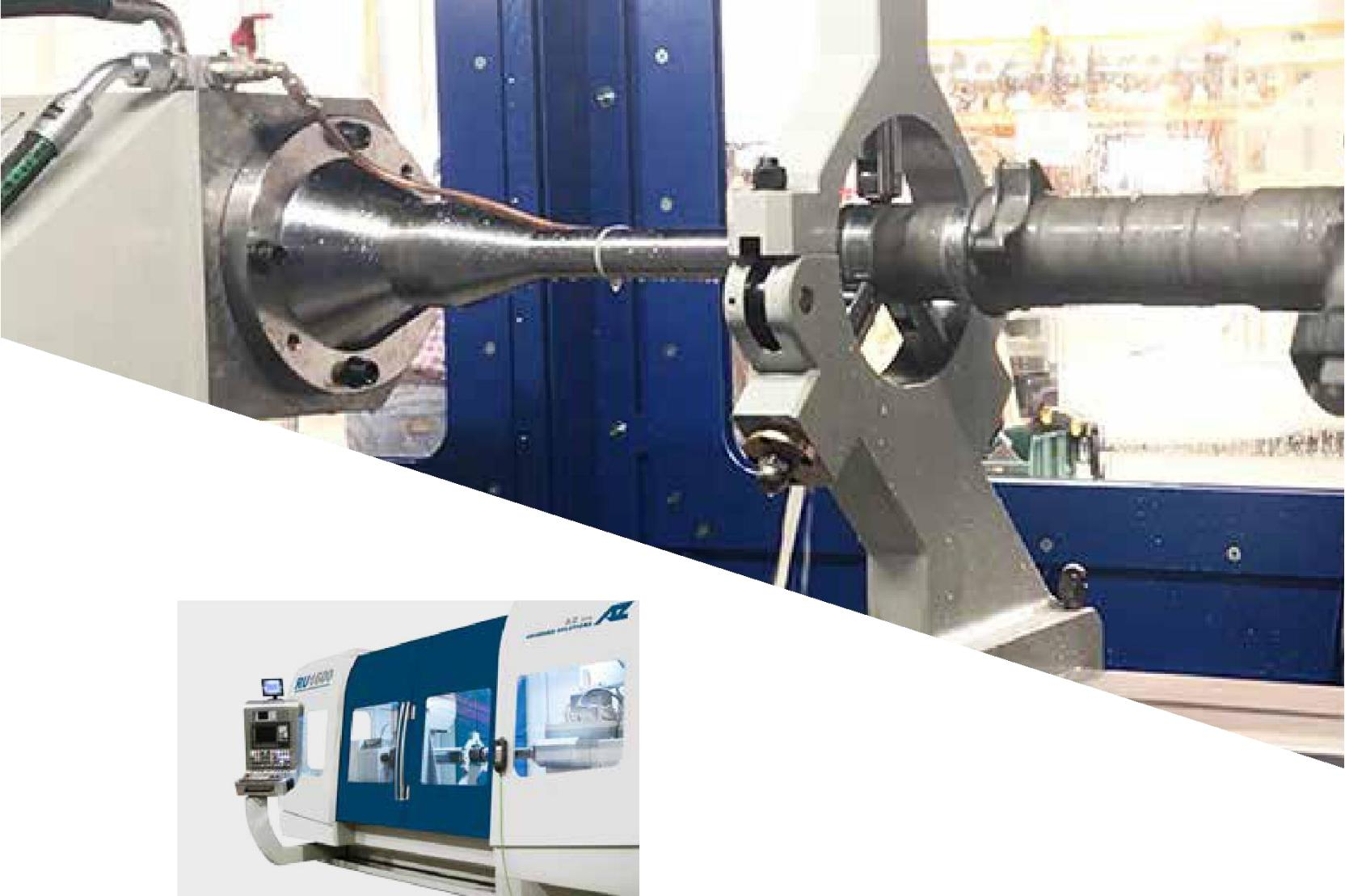
screw system and linear guideways. The workpiece is clamped by headstock and supported by steady rest moves easily on the table. Base is specifically designed to obtain the best result between structural deformations and vibration dumping. The table is realized in two cast iron parts. As optional the table can swivel CNC or manually controlled.
