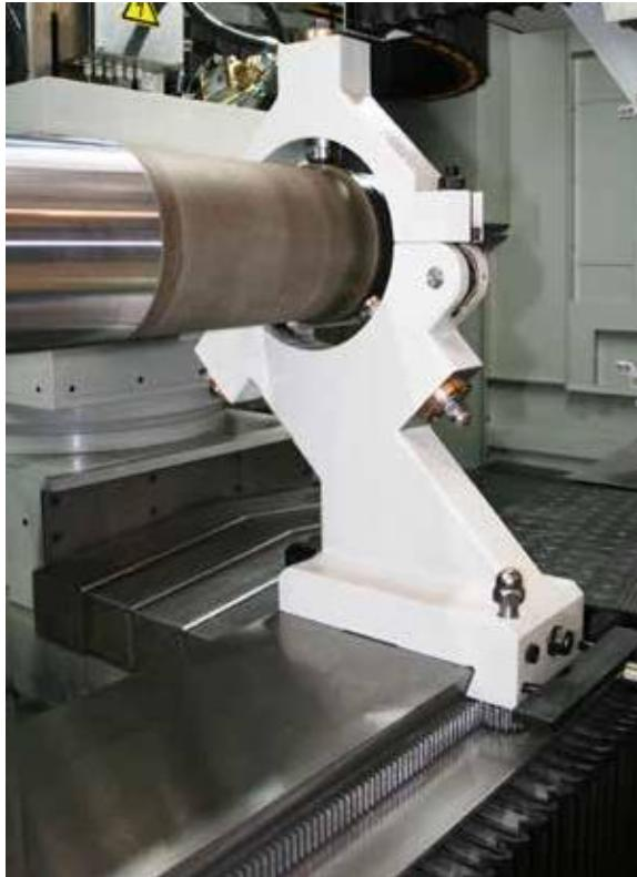
The machine can be equipped with different workpiece supports that can be moved manually or automatically along the table:
