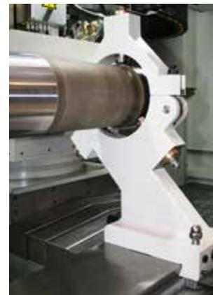
adjustment and continuous control of the force between centers with the possibility of footer pedal control.
