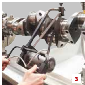
1 Contrappesi supplementari Additional counterweights
