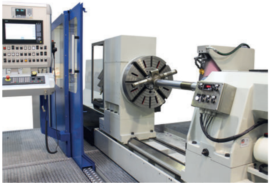
AZ RU universal grinding machines are high performance machines designed to work in the micron range
