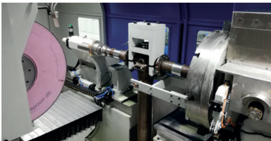
The RU line can be configured to perform the complete machining of landing gear
