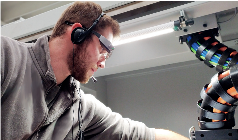
With AZ-SmartGlasses the operator can see notes and components highlighted by AZ with the help of Augmented Reality (AR)
